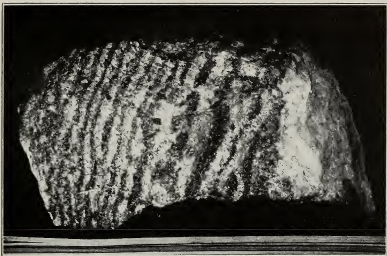
FIG. 12. Banded ore from dump of Cullen Mine near Salem, Kentucky. The light bands are fluorite and the dark bands are sphalerite. They are interpreted as the result of rhythmic deposition during replacement of limestone. Specimen is 10 inches long.
